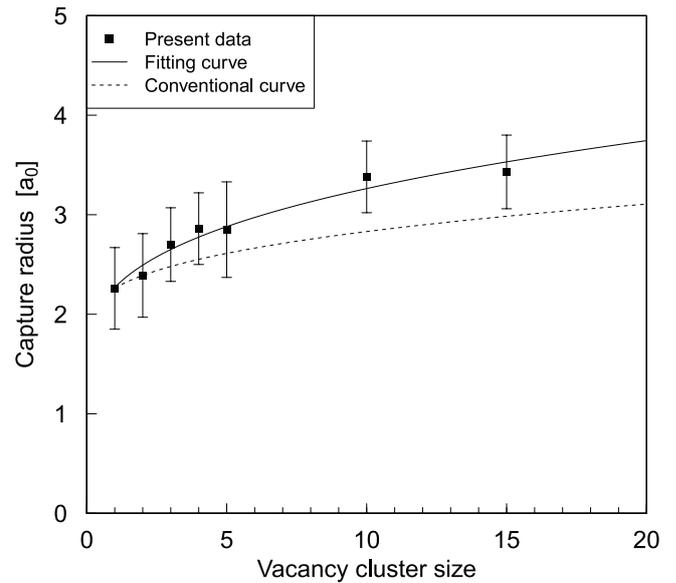
**Figure 5.** Capture radius of vacancy clusters, the fitting curve (1) and the conventional curve (2). Each error bar shows the standard deviation.
