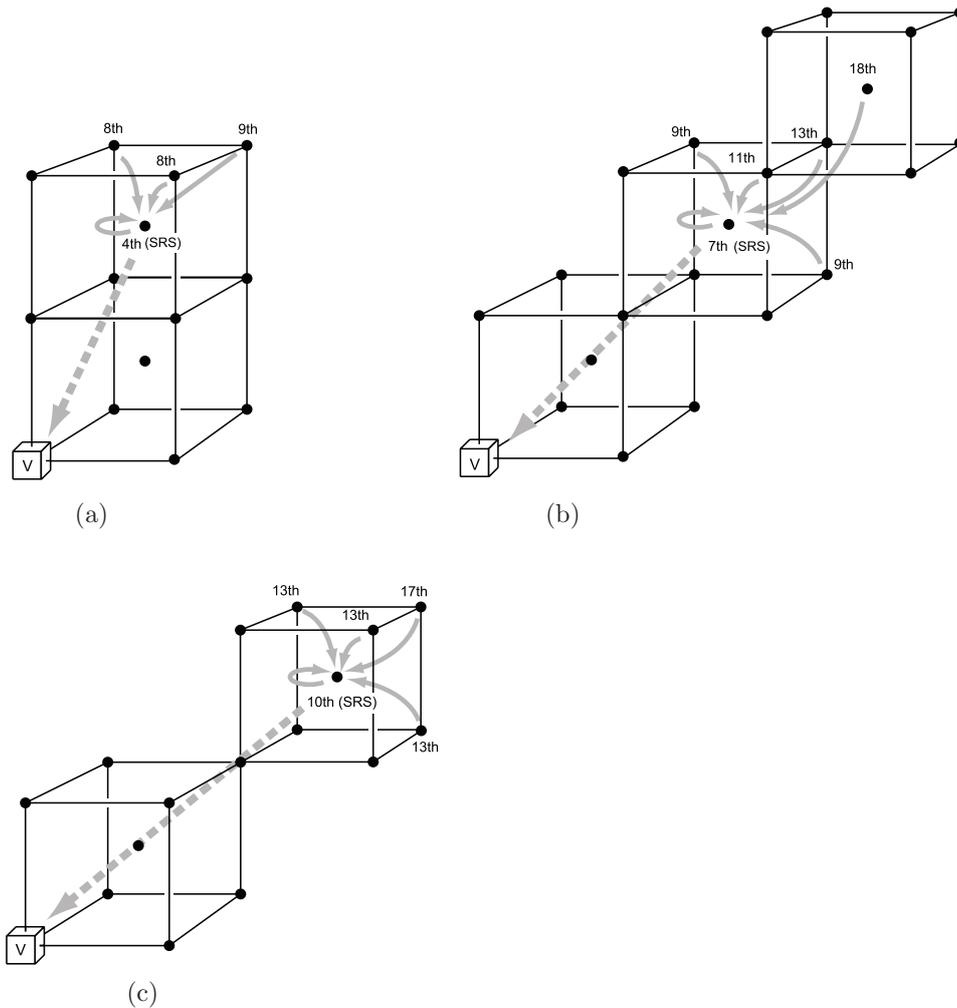
**Figure 3.** The recombination paths where SRS is located (a) at 4th-NN, (b) at 7th-NN, (c) at 10th-NN. Each small cube with the mark V shows a vacancy site. Labels on the site, *n*th, indicate nearest neighbor orders.
