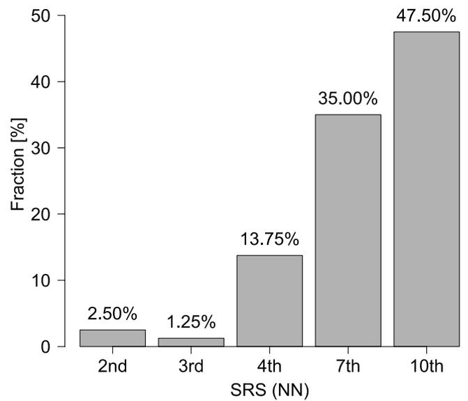
**Figure 2.** Fraction of each SRS for a Frenkel pair recombination. Values obtained by the summation in terms of SRS in table 1.
