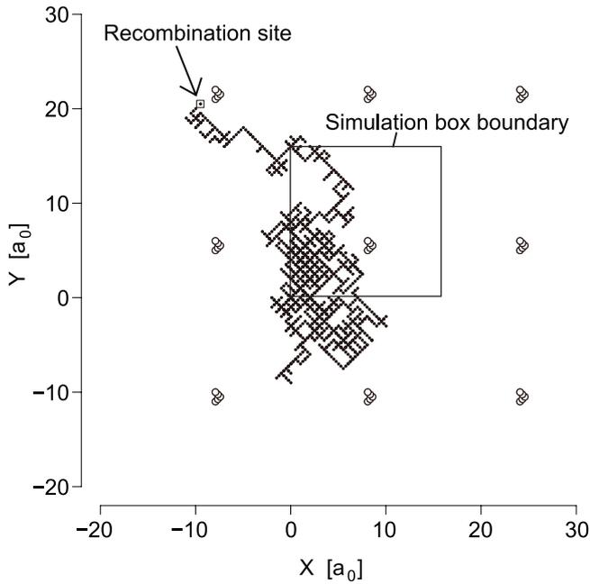
**Figure 1.** Projection of SIA diffusion trajectory on XY plane. Filled dots show SIA positions and open dots show the vacancy positions. The recombination site of the SIA is indicated by a tiny square mark. Phantom images of the vacancy positions are drawn outside the simulation box to depict the effect of periodic boundary conditions.
