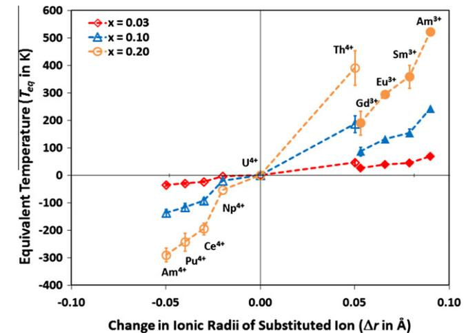
**Fig. 11.** The effect of concentration on the equivalent temperature ( $T_{eq}$ ) for each type of substituted specie in  $UO_2$ . The open symbols are for 4+ ions and solid symbols are for 3+ ions. The magnitude of  $T_{eq}$  increases with an increase in concentration. The error bars are associated with the predicted  $T_{eq}$  for a particular substituted ion with different potentials.
