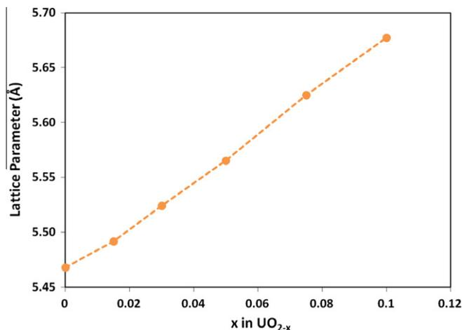
**Fig. 4.** Variation in lattice parameter due to  $\text{U}^{3+}$  ion substitution in  $\text{UO}_{2-x}$  system using Pot3. Pot3 is the only potential which can describe  $\text{U}^{3+}$  ion substitution.
