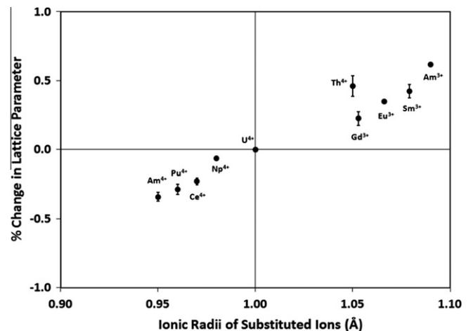
Fig. 8. Effect of 4+ and 3+ ion substitutions in uranium dioxide, where the stoichiometric fraction of A is 0.20. The error bars are the error associated with the predicted lattice parameter variation for a particular substituted ion with different potentials.
