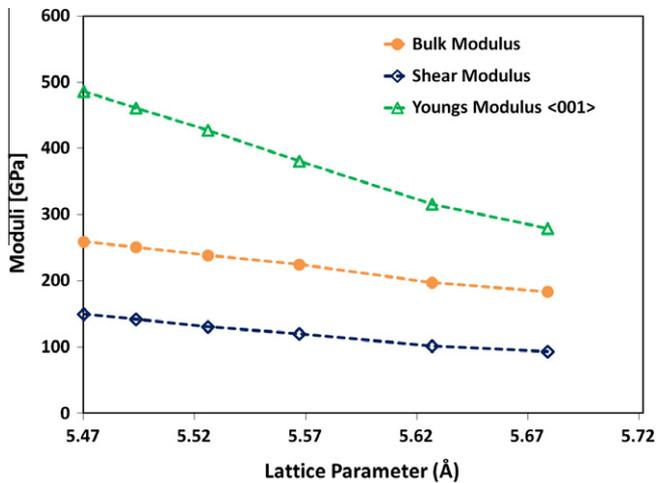
Fig. 5. Variation in bulk, shear, and Young's modulus in  $\text{UO}_{2-x}$  system using Pot3.
