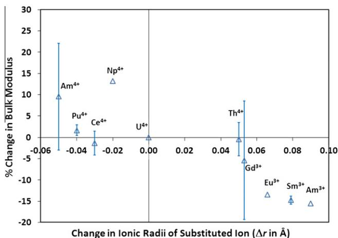
**Fig. 12.** The % change in bulk modulus calculated for each type of substituted specie in  $\text{UO}_2$ . Most of the 4+ ions increase the bulk modulus while most of the 3+ ions reduce the bulk modulus. The error bars are associated with the predicted % change in bulk modulus with different potentials for a particular substituted ion.
