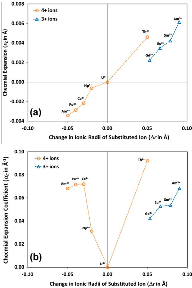
**Fig. 9.** Comparison of (a) chemical expansion ( $\epsilon_c$ ) and (b) chemical expansion coefficient ( $\alpha_c$ ) of 4+ and 3+ ion substitution in  $U_{0.80}A_{0.20}$  system. The ( $\epsilon_c$ ) increases with an increase in the substituted ionic radii with respect to  $U^{4+}$  ionic radius, and vice versa. The ( $\alpha_c$ ) is always positive and increases with the increase in the magnitude of the change in ionic radii.
