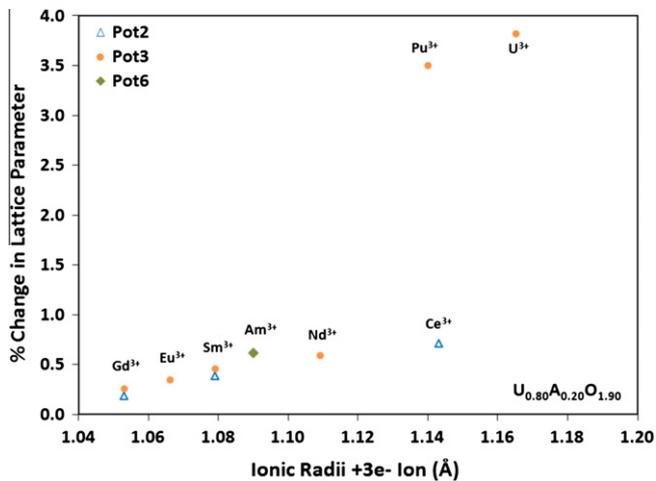
Fig. 6. Variation in lattice parameter due to 3+ ion substitution in  $\text{U}_{1-2x}\text{A}_{2x}\text{O}_{2-x}$  system, where  $2x = 0.20$ .
