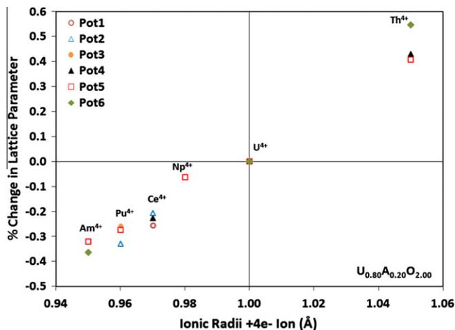
**Fig. 3.** Variation in lattice parameter due to 4+ ion substitution in  $\text{U}_{1-x}\text{A}_x\text{O}_2$  system, where  $x = 0.20$ .
