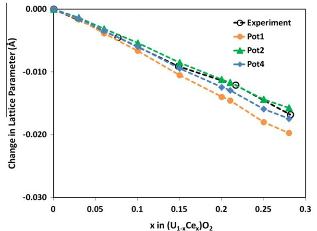
Fig. 2. Relative variation in lattice parameter due to 4+ ion substitution in  $\text{U}_{1-x}\text{Ce}_x\text{O}_2$  system with respect to the bulk  $\text{UO}_2$  lattice parameter.
