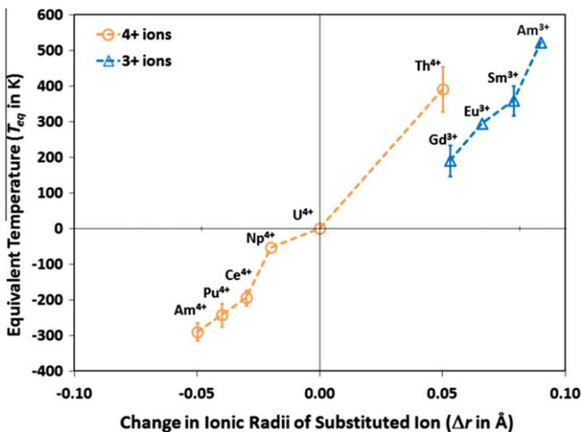
**Fig. 10.** The calculated equivalent temperature ( $T_{eq}$ ) for each type of substituted specie in  $UO_2$  to achieve an equal amount of lattice expansion or contraction in a perfect  $UO_2$  lattice. The experimental linear thermal expansion coefficient was used to derive these temperatures. The error bars are associated with the predicted  $T_{eq}$  with different potentials for a particular substituted ion.
