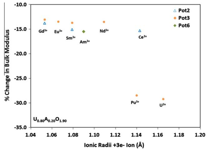
Fig. 7. Variation in bulk modulus due to 3+ ion substitution in  $\text{U}_{1-2x}\text{A}_{2x}\text{O}_{2-x}$  system, where  $2x = 0.20$ .
